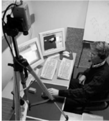
Figure 1. Experimental set-up for generating visual scene and speech input for the system. A video camera views events that are generated by the human operator, who at the same time narrates the ongoing events.
